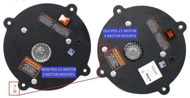
The above image displays the new motor (left) and previous motor (right) attached to the faceplate. Please note that the new motor on the left now has 3 motor mounts, reduced from 4 motor mounts seen on the right. New motors can be attached to existing faceplates with 4 mounting holes by utilizing 3 of 4 mounting points. The 4<sup>th</sup> motor mount on the old faceplate (red square on the right) can be blocked with nuts, bolts, & washers (red square on the left).
