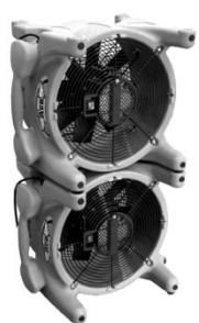
*Stack for Operation* – Set one Ace TurboDryer on its wide feet (handle on the side) on a stable, level surface. Place a second Ace TurboDryer on top so that its rubber feet fit into the impressions on the bottom unit. Always use caution when stacking for operation to avoid damage or injury from a falling unit.
