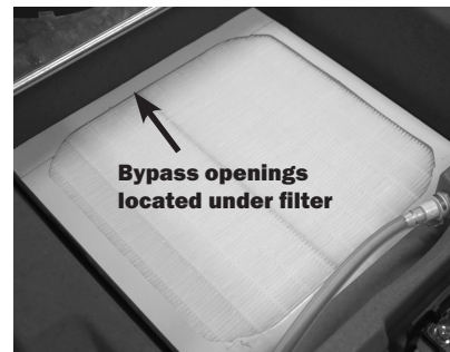
Figure 6: Remove filter, snap grain control cover into position shown, and replace filter.
