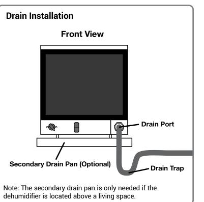
Use care to keep the hose as flat to the floor as possible after your trap is in place. Be sure the hose is not kinked or otherwise restricted so water can pass through the hose freely. Improper installation of the drain hose may result in water leakage.
