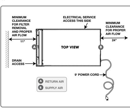
• Electrical service access will require the removal of the outside shell. Allow sufficient clearance around the unit.
