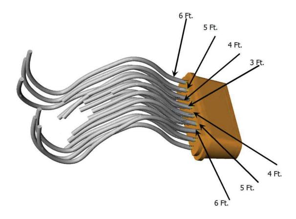
In order to achieve the best air pressure for wall drying, Viking Equipment recommends that the  $\frac{1}{2}$  x  $\frac{3}{8}$  inch Vinyl hoses be cut as shown above. Lengthening hoses will result in a loss of pressure unless pressure is equalized by capping-off one or more hoses to compensate. Hose caps are incorporated into the front of the PDS-21, below the Viking logo.
