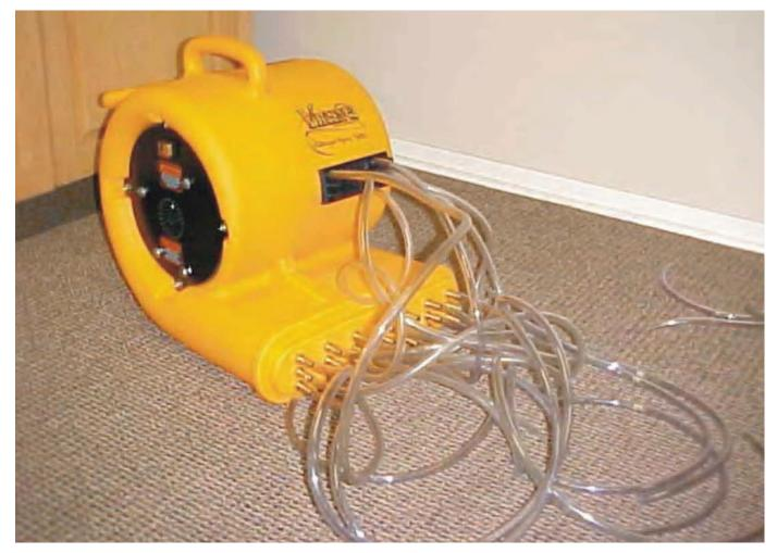
**NOTE\*** END HOSE THAT IS NOT PLUGGED INTO A WALL HOLE MAY BE PLUGGED BACK INTO THE PLUG-OFF SYSTEM ON THE UNIT INCREASING THE AIR FLOW TO THE OTHER HOSES.
